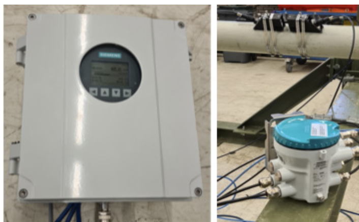
Figure 7: Wide-Beam Sensors FSS200 in 2-path reflect mount, FS230 transmitter and External DSL
